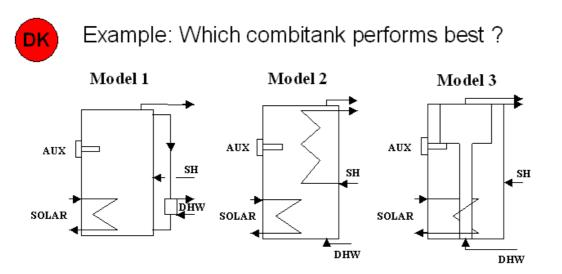
Figure 5 – Denmark: best configuration of DHW preparation is studied through modelling
