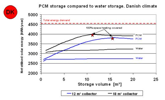
Figure 9 – Denmark: The subcooling effect might be an advantage for seasonal storage according to preliminary simulations
