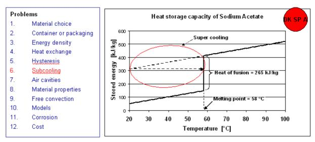
Figure 8 – Main issues of PCM storage and the subcooling effect that must be modelled to accurately predict the performance of a PCM storage
