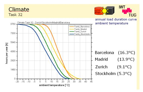
Figure 3 – Four climates are considered in Task 32 to evaluate different storage designs in solar combisystems
