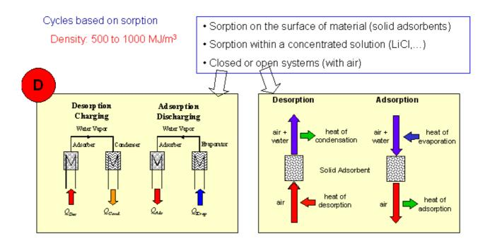
Figure 10 – Germany: Principle of a sorption storage in closed (left) or open (right) systems during charging and discharging phase
