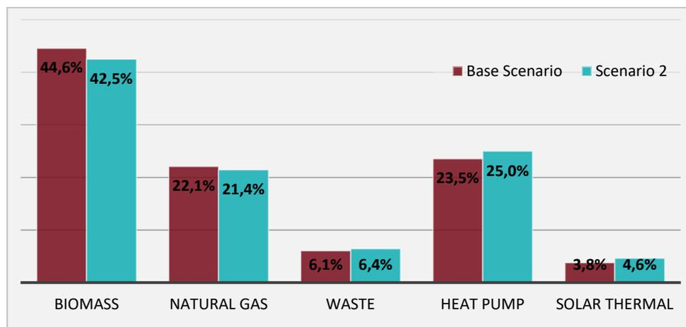
Figure 3: Sensitivity analysis of district heating generation in Austria (base scenario vs scenario with 20% higher price for gas and biomass)
