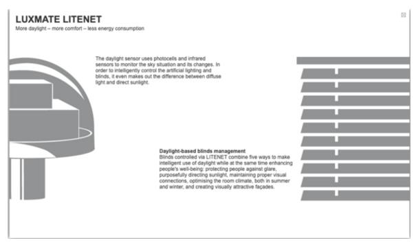
The outdoor sophisticated sensor tracks the power and the directionality of available daylight, and 5 options of blind positions are proposed to make the facades more homogeneous.
