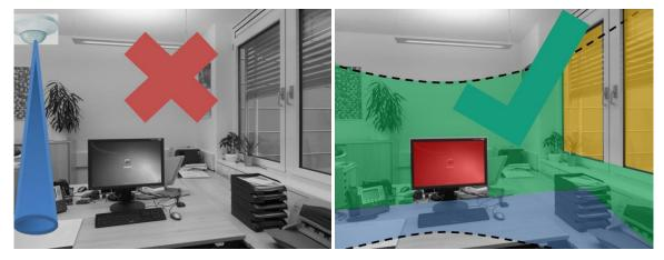
Conventional lighting controls detect and regulate horizontal illuminance levels (left), but the user comfort is predominantly in the vertical field of vision(right). © Fraunhofer IBP
