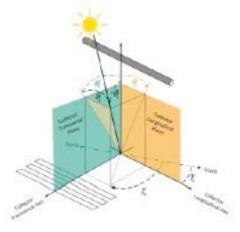
Transversal and longitudinal directions and plans of the collector (hofer et. al. 2015a. Comparison of Two Different (Quasi-) Dynamic Testing Methods for the Performance Evaluation of a Linear Fresnel Process Heat Collector. In: Energy Procedia (69), S. 84–95).
