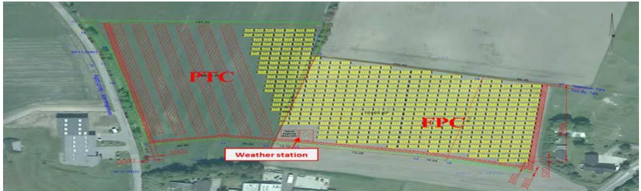
Fig. 3 Layout of the hybrid solar collector field in Taars (Source: Aalborg CSP A/S).
