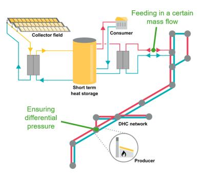
Figure 3: Scheme of a DH network with one decentral feeding point
