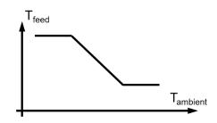
Figure 1: Typical adjustment of the feed temperature to the ambient temperature
