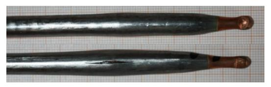
Figure 3: Heat pipes after freeze resistance test (Source: HPQUAL - Investigation of freeze resistance testing of heat pipes; Fraunhofer ISE)
