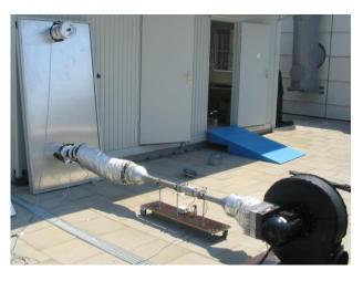
Figure 1: Test setup including a fan, a volumetric flow meter and an electrical pressure gauge at TestLab Solar Thermal Systems, Fraunhofer ISE.
