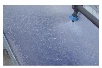
Figure 1: External Thermal Shock Test; Fraunhofer ISE
