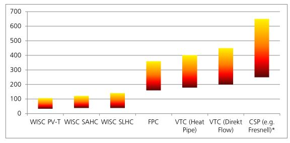
Figure 2: Attainable range of standard stagnation temperatures for different collector technologies. (Source: Fraunhofer ISE) \*Stagnation is avoided by defocusing for CSP because temperatures can be too high
