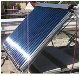
Figure 1: Internal thermal shock test; Fraunhofer ISE
