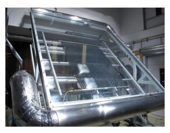
Figure 1: Internal pressure test of a polymeric collector at the indoor solar simulator of the TestLab Solar Thermal Systems, Fraunhofer ISE.
