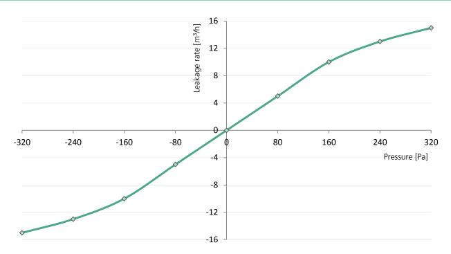
Figure 2: Typical Leakage rate curve fitted with a 3<sup>rd</sup> order polynomial on the basis of flow measurement points for positive and negative pressures.
