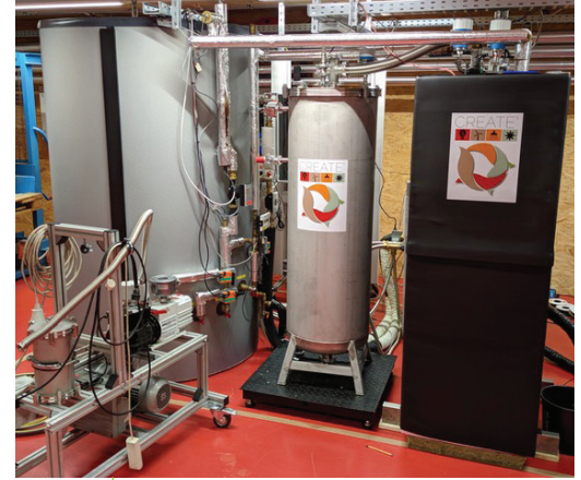
▲ Laboratory test set-up of the prismatic heat battery (to the right) and the evaporator/condenser (middle). Source: AAE INTEC
