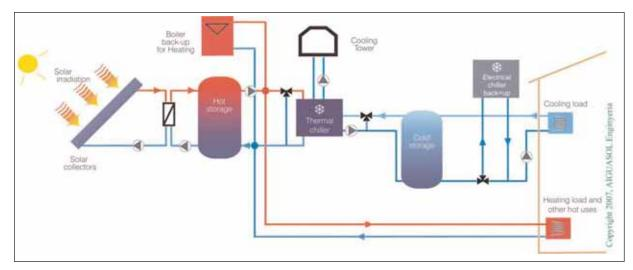
A schematic of a solar combi+system. (Source: AIGUASOL)
