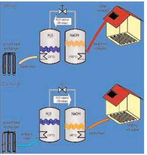
A schematic of NaOH storage.
