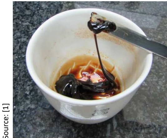
D-mannitol after 166 h melted under air @180 °C
