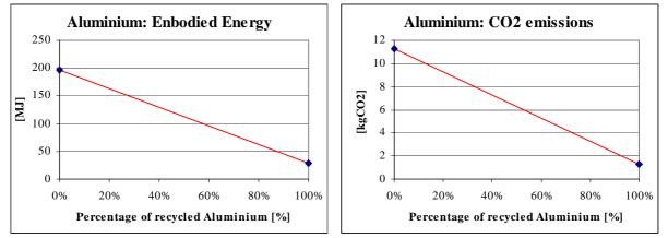
Fig. 3: Embodied energy and  $CO_2$  emissions for variable percentages of recycled aluminium in the aluminium sheet
