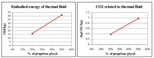
Fig. 2: Embodied energy and  $\text{CO}_2$  emissions for variable percentages of glycol in the thermal fluid
