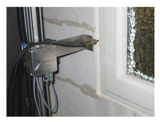
Figure 5.2: The humidity sensor mounted on the scanner
