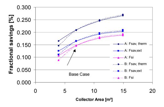
Figure 6: Control strategy A: Boiler running all year, B: Electric immersion heater used in summer
