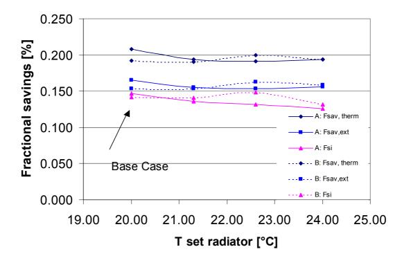
Figure 12: Variation of Set temperature radiator thermostat summer. A: Radiator thermal mass 1,150 kJ/K, B: Radiator thermal mass 11,500 kJ/K
