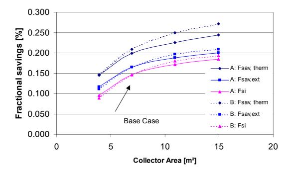
*Figure 10: New control strategy that always have collector to run at lowest temperature. A: New strategy, B: Base case Strategy*
