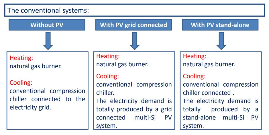
PV systems are sized to generate the electricity required by the chiller and the auxiliaries.
